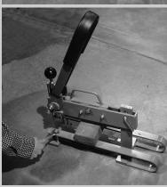
4. Next, adjust the Tension Knob so that the top blade is flush with brick. Push down the handle by using the black rubber covering on the handle to split the brick.
