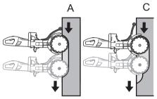
Follow the same saw cut, but further in the work piece (C), and repeat the work with the crowbar.
