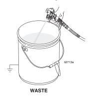
11. Release trigger, engage trigger lock.
