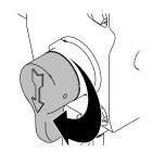
5. Engage trigger lock. Remove tip and guard from gun and place into waste pail for further cleaning.
