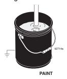
Trigger gun into waste pail until paint comes out of gun. Release trigger, pump will build up pressure and motor will stop. Move gun to paint pail and trigger for 20 seconds.
