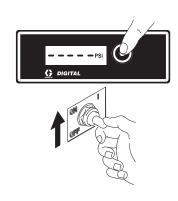
3. **S/N** displays for 1 sec, then the serial number. Short press DTS button. Total motor run hours displays.
