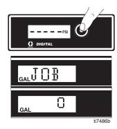
4. Press and hold to reset to zero, or short press DTS button to move to Lifetime Gallons (or Liters x 10).
