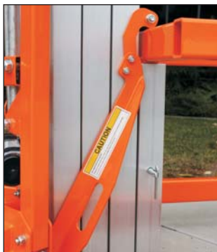
Hold down can be actuated when stabilizers are stowed.
