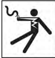
Electric shock resulting in death can occur if you plug this machine into an improperly wired outlet. If the ground wire is electrified, you can be electrocuted by just touching the machine, even when the power switch is off. A ground fault circuit interrupter will not protect you in this situation. Use a UL listed tester to determine if the outlet is safe.
