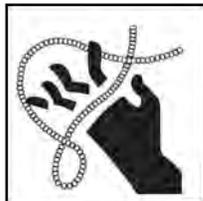
Do not overstress cables. Overstressing cables may cause twisting, kinking, or breaking of the cable and may result in serious injury.
