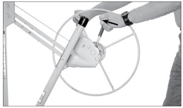
3. To lower the PANELLIFT® Drywall Lift control the backward rotation of the winch by grasping the winch handle with your right hand BEFORE releasing the brake with your left hand. ALWAYS use this two hand method when lowering the PANELLIFT® Drywall Lift.
