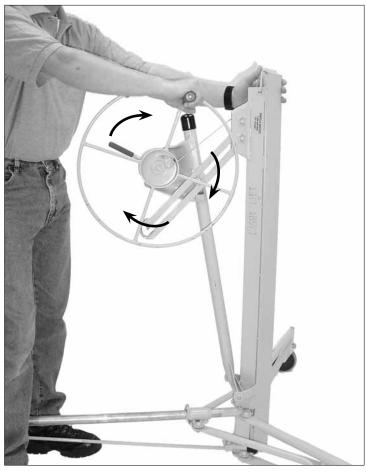
8. Hold the retaining hook in this position with your left hand and rotate the winch forward with your right hand. This will cause the winch assembly to fold up against the frame. When the slide bar contacts the frame, tighten the cable just sufficiently to hold the winch in the collapsed position.
