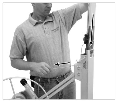
6. Pull the slack cable through the sheave pocket and slide the telescoping sections into the frame housing.
