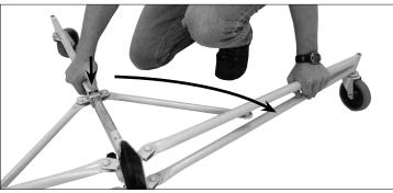
1. Begin by setting up the tripod base: press down on the slide yoke pin clip and swing the outer legs out until they lock in the working position (note the holes on the bottom of the slide tube).
