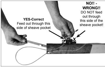
8b. Repeat the process performed in steps 2 - 3: Insert the crimped end of the cable up into the end of the sheave pocket at the end nearest the bottom of the "B" section as traced by the dotted arrows. Twist the installation tool while holding the crimped end of the cable up into the sheave pocket. Pull the crimped end out completely to remove the slack.
