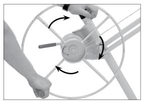
2. To raise the PANELLIFT® Drywall Lift rotate the winch wheel in the direction shown. The brake arm is spring loaded to hold the winch automatically at any height.
