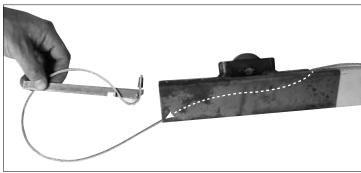
8a. Reload and insert the cable installation tool into the BOTTOM end of the "B" section as shown.
