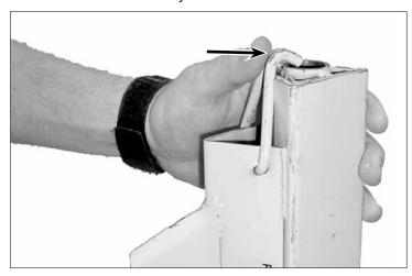
7. With the telescoping section all the way down, position the retaining hook over the top as shown.
