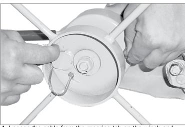
1. Loosen the cable from the mooring tab on the winch and pull it out from the winch drum. BE CAREFUL! A worn cable can have frayed strands. Wearing gloves will help protect your hands.
