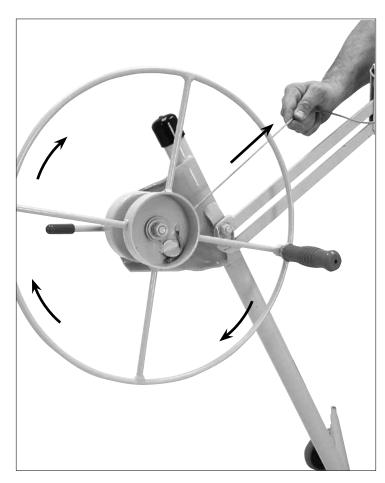
7. Feed the cable through the winch drum and secure it firmly behind the mooring tab as shown. Rotate the winch wheel in the direction indicated to take up the slack in the cable.
