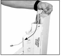
4. Feed the crimped end of the 186-00 cable through the frame sheave pocket from the top. It is VERY IMPORTANT that the cable passes OVER THE TOP of the cable sheave as shown here.
