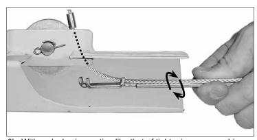
6b. With a clock-wise motion like that of tightening a screw driver, twist the cable installation tool while holding the crimped end of the cable up into the sheave pocket. The cable will pop loose from the tool and pop up through the sheave pocket as shown in this cut away view.
